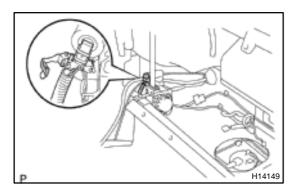
(b) Disconnect the pretensioner connector as shown in the illustration.
